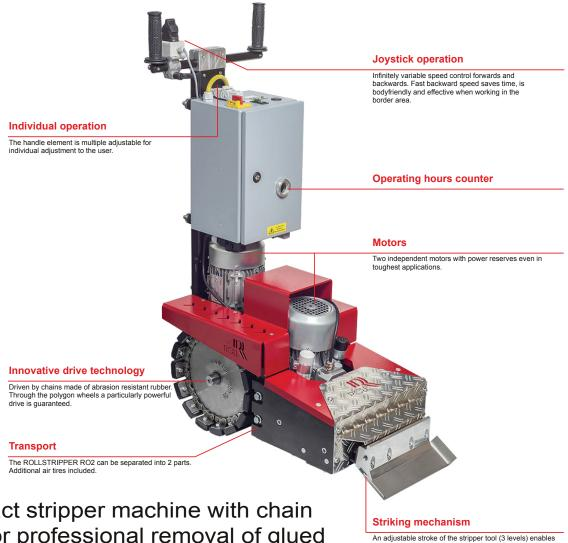
Compact stripper machine with chain drive for professional removal of glued floor coverings such as parquet, carpeting, linoleum, PVC and vinyl.
